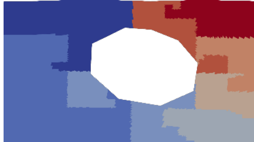
Figure 6: The 2D mesh partitionned using an Hilbert curve.
