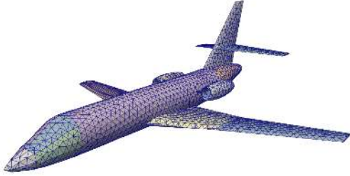
Figure 18: FEM surface mesh of the Falcon, showing elements not complying with the user-defined spacing.
